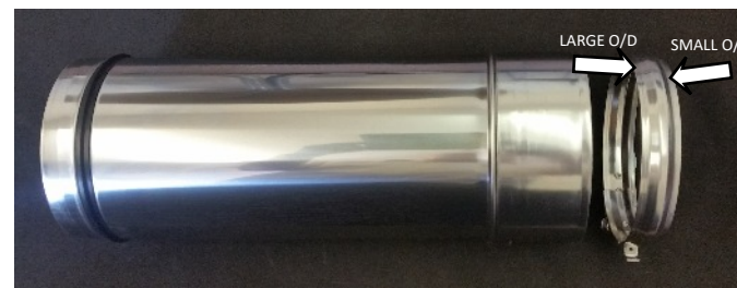
7. LOCKING BAND ASSEMBLY - FIT THE LARGER DIAMETER OF THE BAND TO THE SOCKET / FEMALE END.
