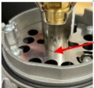
Ensure diffuser support fits through air distributor plate
